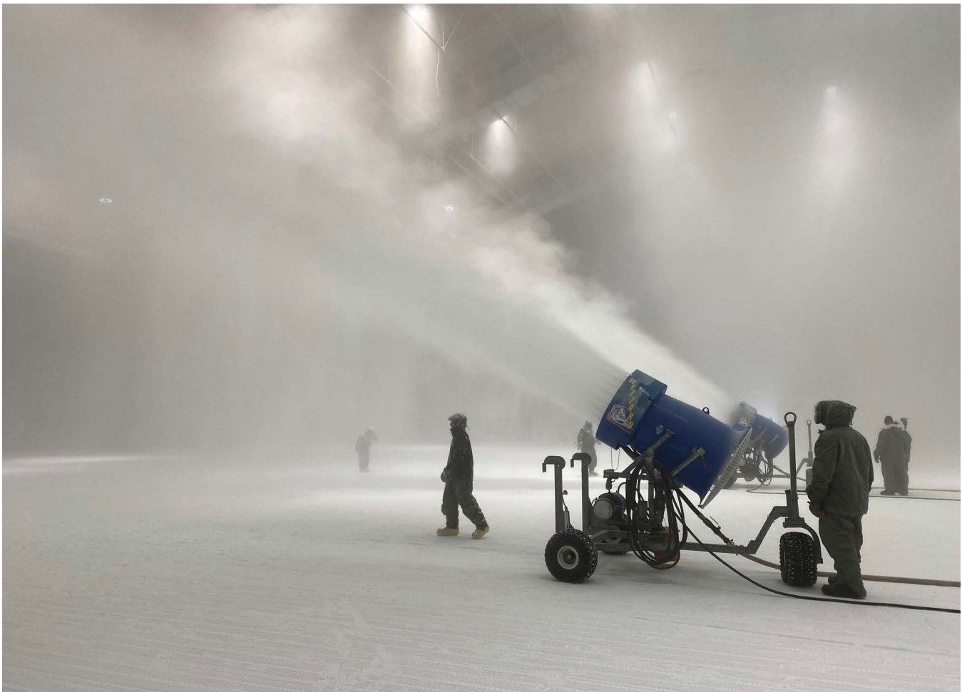
Team members at the McKinley Climatic Laboratory at Eglin Air Force Base, Florida, use machines to create snow to prepare for environmental testing.
